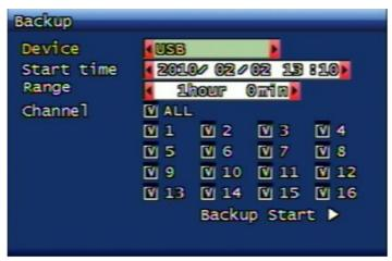
DVR-RW • It starts backup processing of video data onto the relevant backup device (CD or DVD disc) from HDD when the DVD-RW driver is equipped and CD/DVD discs are inserted by using Backup menu. • It starts backup processing within the capacity of CD or DVD disc when selecting Backup menu > Backup time selection > Backup start. • By carrying SimplePlayer program with backed-up Media, the user can execute the playback at any time. • The backed-up files can be played back on
